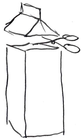
④ CUT A 12mm WIDE SECTION OF THE TUBE YOU ARE USING. USE A FINE TOOTHED SAW & CUT THIS SECTION AS ACCURATELY AS YOU CAN. USE A MITER BOX IF YOU HAVE ACCESS TO ONE.
